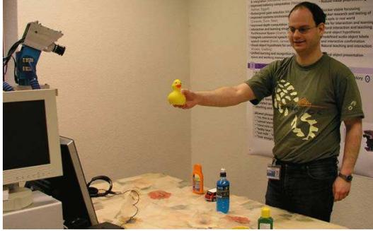
Fig. 7. The online learning scenario for recording training and testing images. Objects are shown freely by hand and a gaze control system using disparity focuses on the objects that are in the peripersonal space between user and the camera.
