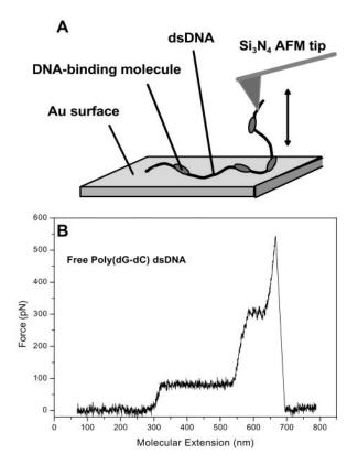
FIGURE 1 (A) Experimental setup; (B) Force-extension trace for free poly(dG-dC) dsDNA.
