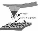
FIG. 2. Scheme of the immobilization concept. The antigen fluorescein is covalently bound by means of a poly(ethylene glycol) linker to the silanized silicon nitride AFM tip. Single-chain Fv'-fragments (scFv) of an anti-fluorescein antibody are attached directly to a gold surface by an engineered C-terminal Cys residue. The black ovoids on the surface represent the protection layer of negatively charged thiol compound needed to avoid denaturation of proteins on gold.
