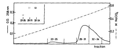
Figure 6: Elution of 0.3 mg of an endo R.EcoR I digest of plasmid pGM 214 (20) DNA from a malachite green column: 1.5 x 16.0 cm, 5.8 ml/hr flow rate at room temperature.
