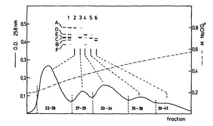
Figure 7: Elution of 0.45 mg of lambda DNA digested by endo R.EcoR I from a malachite green column:  $1.5 \times 16$  cm, 5.8 ml/hr flow rate at room temperature.
