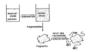
Figure 1: Scheme of the 'two step polymerization procedure' for synthesis of a novel material for affinity chromatography of nucleic acids.
