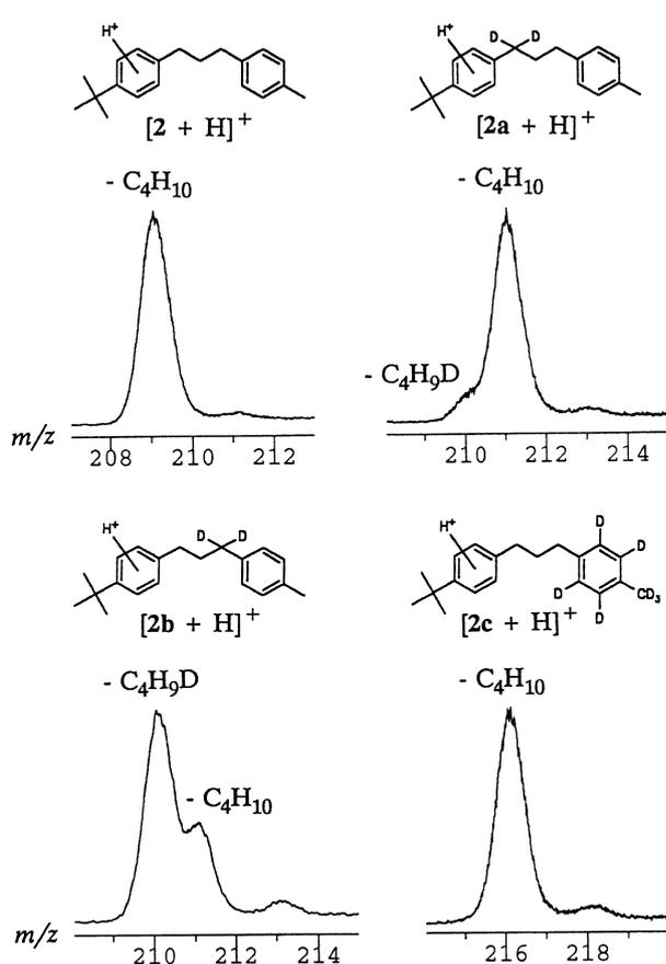
**Figure 1.** Partial MIKE spectra of  $[M + H]^+$  ions of **2** and deuterium labelled analogues **2a–2c**. Note that contributions at  $m/z$  211 (**2**),  $m/z$  213 (**2a** and **2b**) and  $m/z$  218 (**2c**) correspond to the fragmentation of molecular radical ions  $[M^{\bullet+}]$  which contain naturally occurring  $^{13}\text{C}$ .
