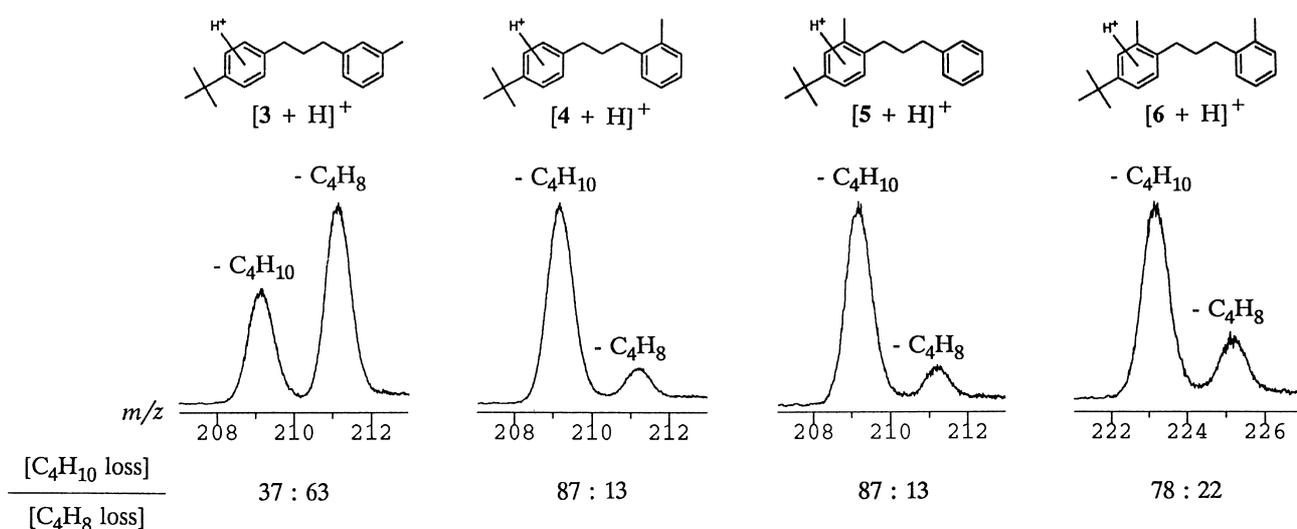
Figure 3. Partial MIKE spectra of  $[M + H]^+$  ions of methyl substituted precursors 3–6 (for ions  $[2 + H]^+$ , see Figure 1).
