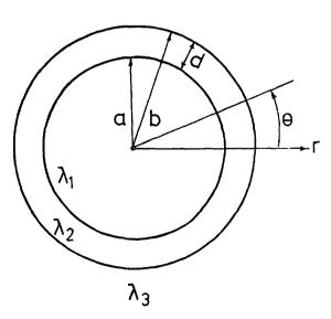
Fig. 1. Scheme of a diametral cross-section through a spherical vesicle; a and b are the inner and outer radii, respectively, of the membrane shell. E is the electric field vector and  $\lambda$  denotes the conductivity
