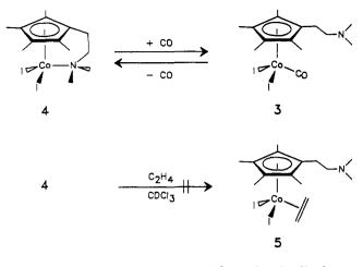
dark purple. The carbon monoxide molecule displaces the dimethylamino group; this leads to the formation of carbonyldiiodo( $\eta^{5}$ -1-[2-(N,N-dimethylamino)ethyl]-2,3,4,5tetramethylcyclopentadienyl)cobalt(III) (3).
