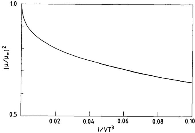
Fig. 2. Volume dependence of the Debye mass from continuum perturbation theory in a finite box. Shown is the square of the ratio  $\mu/\mu_\infty$  between the Debye mass in a finite and in an infinite volume, as function of  $1/VT^3$ .
