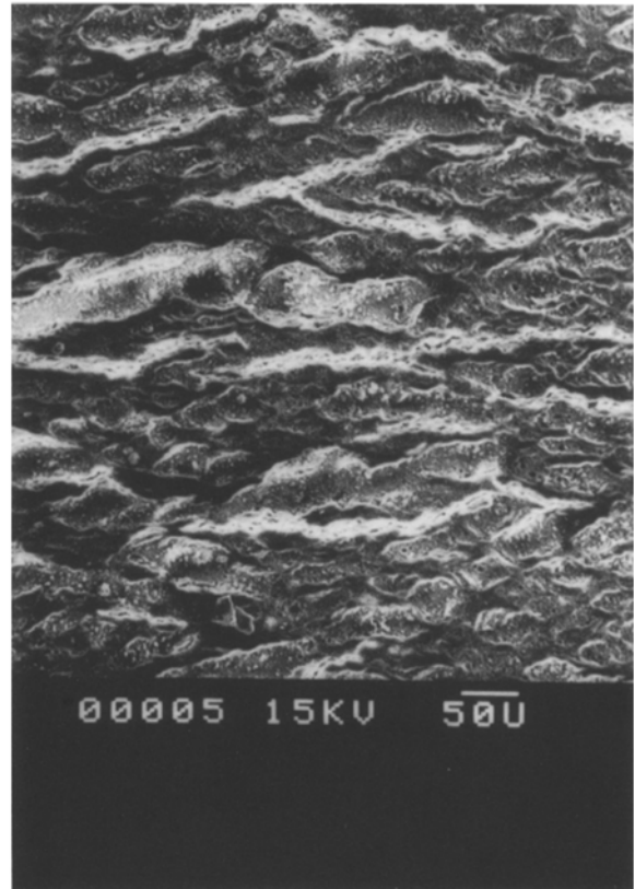
Fig. 6b) PP membrane after long term perfusion culture.
