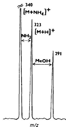
Fig. 4. MIKE spectrum of  $[M + \text{NH}_4]^+$  ion of 3-fluoro derivative 2.
