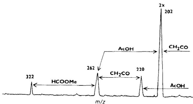
Fig. 3. HV spectrum of 4-fluoro derivative **3**, showing pathways to ions having  $m/z$  160.
