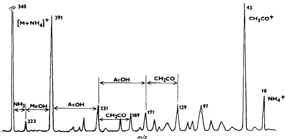
Fig. 5. CID spectrum of  $[M + \text{NH}_4]^+$  ions of 3-fluoro derivative 2.
