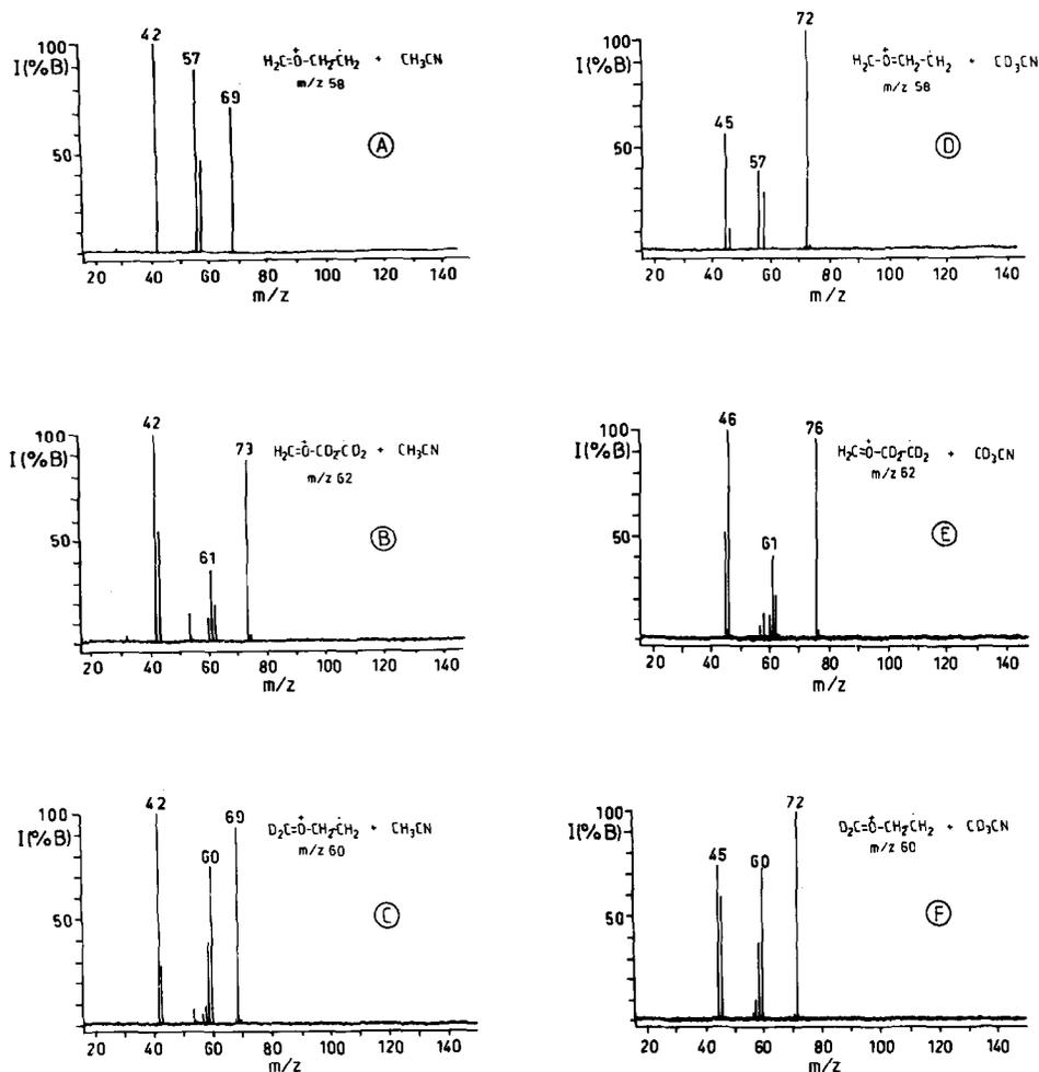
Fig. 2. Bimolecular reaction of the  $\beta$ -distonic ion with acetonitrile and acetonitrile- $d_3$ : (A) and (D), a; (B) and (E), b; (C) and (F), c. Mass spectra were obtained after 1 s reaction time. Total pressure,  $5.0 \times 10^{-8}$  mbar; background pressure,  $(0.5-1.0) \times 10^{-9}$  mbar.
