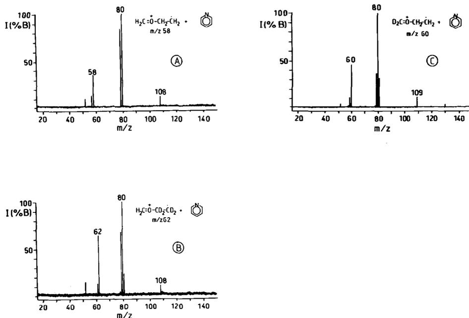
Fig. 1. Bimolecular reaction of the  $\beta$ -distonic ion with pyridine: (A), **a**; (B), **b**; (C), **c**. Mass spectra were obtained after 1 s reaction time. Total pressure,  $5.0 \times 10^{-8}$  mbar; background pressure,  $(0.5-1.0) \times 10^{-9}$  mbar.
