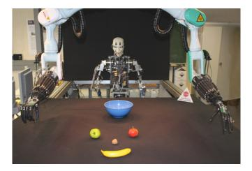
Fig. 1. The current Curious Robot Interaction Scenario. Two Mitsubishi PA-10 robot arms are fixed to the ceiling, with a left and right Shadow robot hand attached. In the background, an anthropomorphic robot torso is present. Sensors not visible are an overhead camera and a headset microphone.
