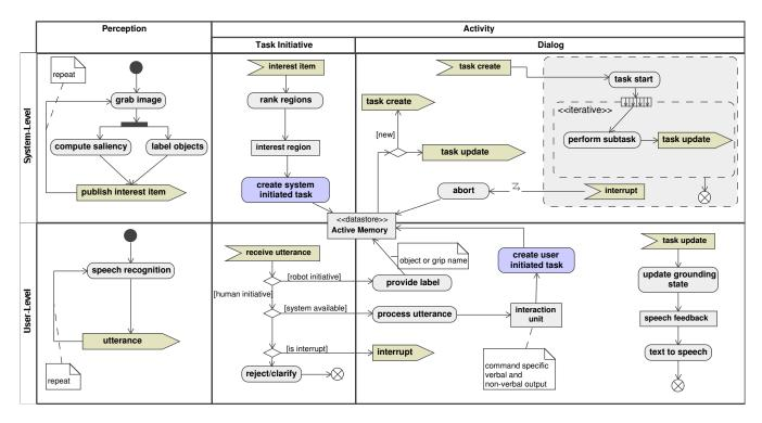
Fig. 2. UML 2.0 System Activity Diagram. Note that components execute in parallel and communicate using event signals, facilitating extensibility in the proposed system. Different input modalities are mapped to different task types to realize mixed-initiative.
