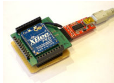
(c) Handmade board with manufactured XBee Carrier Board
