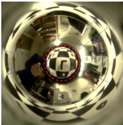
Figure 4. Example of a camera image used for estimating the translation \vec{t}^{\text{ml}} and rotation \vec{w}^{\text{ml}} between the reference frames of the inner and outer image part (see text for details). Corner points in both image parts corresponding to the same point on the pattern are connected by dashed lines. The dashed circle marks the boundary between the inner and outer image part.
