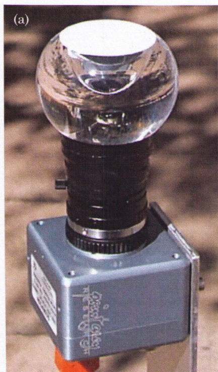
Fig. 1. (Color online) Overview of the new panoramic imager. (a) Picture showing the imaging arrangement mounted on a firewire video camera (1/2" CCD sensor) with an off-the-shelf 6 mm C-mount lens. The Perspex block can be attached to the filter thread of the camera lens. (b) Vertical transect and ray tracing for the new sensor. The surface of the clear Perspex is shown as a bold curve. The red curve shows where the Perspex is coated with a thin reflective surface. Through a central hole in the coating, rays are refracted at the curved surface of the Perspex and by a plano-concave lens.
