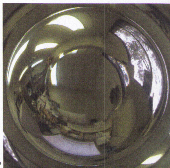
Fig. 9. (Color online) Imaging properties of the uncoated Perspex. (a) Ray tracing diagram showing the refraction of the rays in the image center and total internal reflection in the outer part of the image. (b) Setup used to test the uncoated sensor. An earlier version of the vision sensor with exact spherical shape was used. The part of the sphere that does not contribute to the image is covered with black tape to eliminate unwanted internal reflections. (c) Camera image showing the total internal reflection (camera oriented toward a computer keyboard). (d) Image that shows the small overlap between central and outer image parts more clearly. Note the part of window frame that is imaged twice on the right side.
