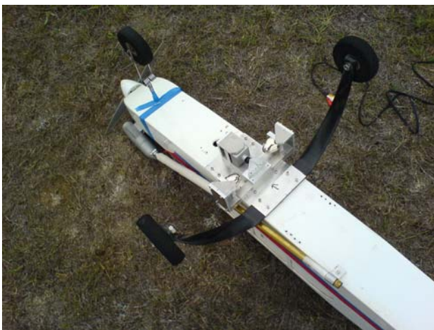
Fig.10. View of system mounted on a model aircraft. The camera faces backwards, but the imaging system captures a frontal view.
