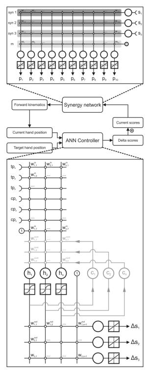
Figure 1: Control schema with inserts showing the synergy network (top insert) and two ANN controller variants (bottom insert). Black structures only: two-layer feedforward network. Black and gray structures combined: recurrent Elman network. For clarity, the number of hidden units is set to 3 ( $h_1$  to  $h_n$ ).
