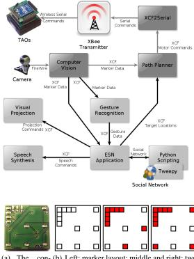
Fig. 2 This collaboration diagram describes the flow of information between the processes in our modular software architecture. The base modules used in this application are shown in dark gray, whereas the new modules are shown in light gray.
