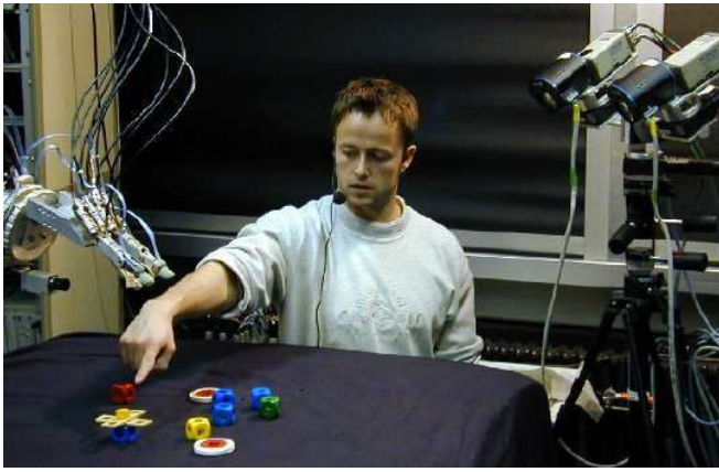
Fig. 1. Interaction with the robot system using speech and gesture. On the left the modified three-fingered TUM Hand is shown.
