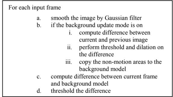
**Figure 2. The background detection and subtraction algorithm**
