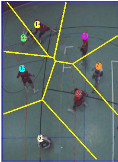
Figure 4. The Voronoi Partitioning used in multiple tracking
