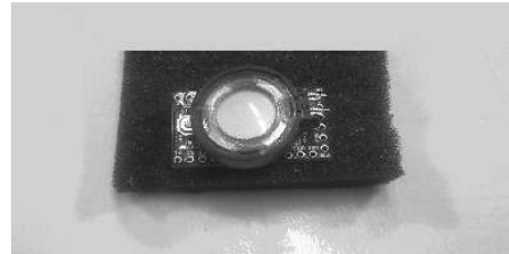
Figure 5: Wearable PCB with loudspeaker
