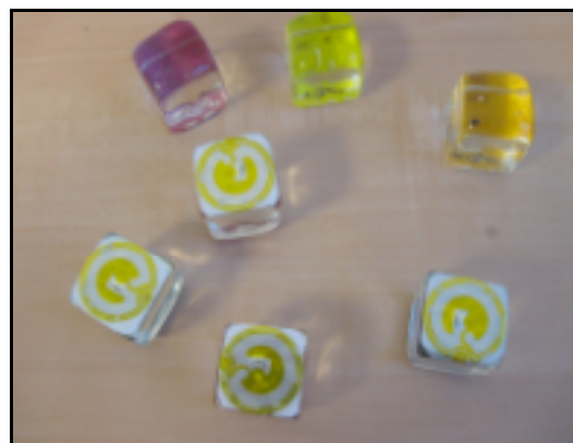
Figure 2. RFID tags under cubic objects.
