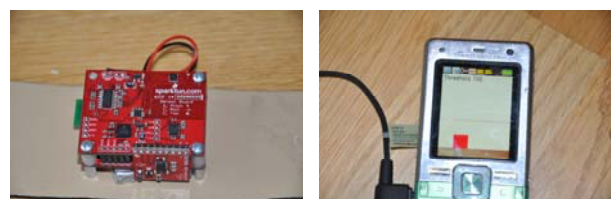
Figure 2. The sensor (left image) used in this experiment. It is a 6DOF (Sparkfun Inc.) inertial measurement unit with Bluetooth antenna. The telephone (Sony Ericsson 650i) received the data via Bluetooth, computed vertical displacement and step frequency and presents the information visually (right image) and via an auditory display.
