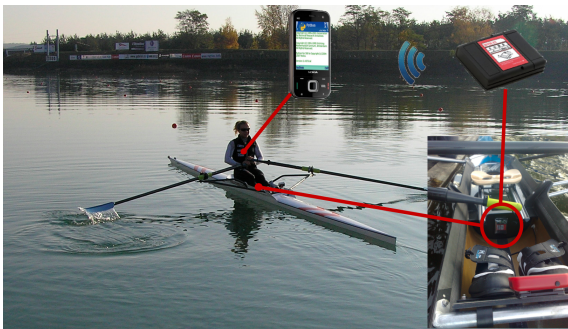
Figure 1: Equipment: the rower carries a smartphone that receives GPS and accelerometer data used for the sonification.
