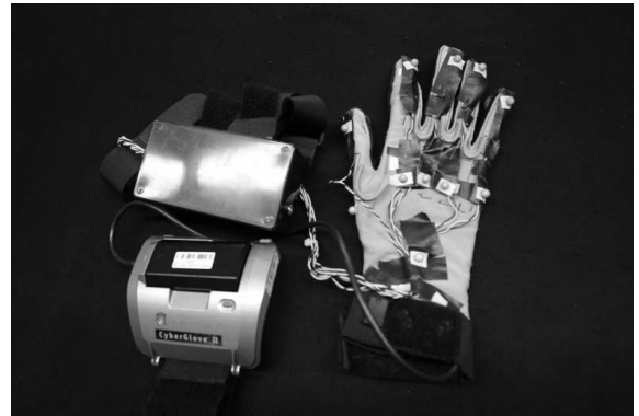
Figure 3. CyberGlove with 11 VICON markers; five markers are situated on the fingertips, five markers on the knuckles and one marker on the back of the hand.
