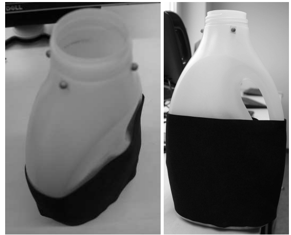
Figure 2. Test object: a large flexible plastic bottle with three VICON markers attached to its neck; 3D positions of the three tracked markers are used for calculating the bottle’s orientation.
