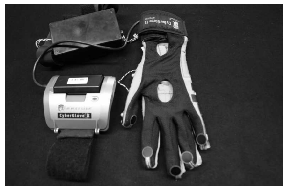
Figure 4. CyberGlove with the integrated TouchGlove: five FSR sensors are fitted on the fingertips.
