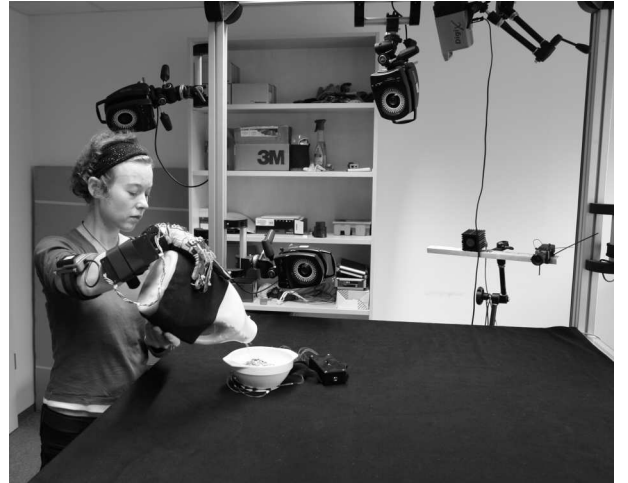
Figure 8. Action capture; while pouring we adjust the orientation of the test object; the content of the test object gradually fills the bowl placed on the scales; the shape of the test object changes as it loses its content due to its changing elasticity.
