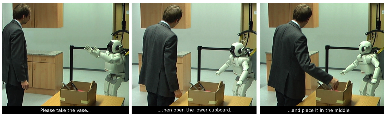
Fig. 12 Example of a multimodal three-chunk utterance delivered by the robot during interaction. Three different types of gesture are used (left to right): iconic gesture illustrating the shape of the vase; pantomimic gesture conveying the act of opening the cupboard; deictic gesture pointing at designated position [37].
