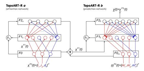
**Fig. 2.** Structure of TopoART-R. Like TopoART, TopoART-R encompasses two modules (TopoART-R *a* and TopoART-R *b*) sharing the input layer *F*0. But the connections of the F2 neurons can either be traced back to  $\underline{i}$  or to  $\underline{d}$ . Furthermore, TopoART-R *b* has an additional input control layer (*F*0<sub>m</sub>) that is required for prediction.
