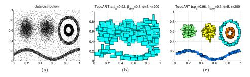
**Fig. 1.** Input distribution and clustering results of TopoART. After presenting each training sample of the dataset (a) to a TopoART network, it created a noise-free representation at two levels of detail. While only one cluster was formed by TopoART a (b), TopoART b distinguishes five clusters reflecting the data distribution in more detail (c). The categories associated with the same cluster share a common colour.
