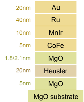
Figure 32: Layer stacking of the full tunnel junctions for all investigated different Heusler compounds.
