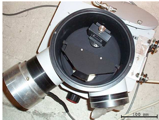
Figure 8.29: Top view photograph into the monochromator.
