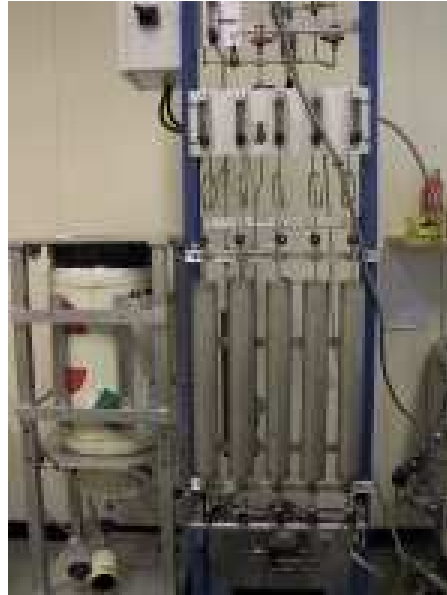
Figure 8.22: Pre-cleaning Setup 2001. The system consists of a special mount for a bottle and a rack with the filter cartridges, a magnetic gear pump (bottom) and a distribution panel with flow meters (top).
