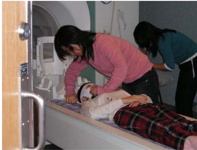
Figure 17: Experiment set-up; the tightly fitting, thermally molded, plastic facial mask which extended from the hairline to the chin was used to avoid a head motion.
