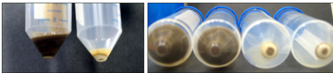
Figure 36 Two different perspectives on freshly prepared haze (24 x 0.5 L Pilsener beer bottles). The larger brown pellet was prepared from a 6 years old beer standard, whereas the white pellets were found in two year old beer.
