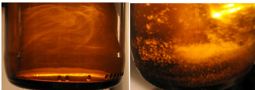
Figure 5 Haze at the bottom of a bottle: a.) chill haze after about 4 weeks of storage at 0 °C (left) and b.) permanent haze after longterm cold storage at 0 °C (right). Chill haze is a reversible type of haze that dissolves again after warming to room temperature. The particles range from 0.1 to 1 \mu\text{m} in size and their control is important as they are regarded as inducers of permanent haze. The enormous amorphous haze here is a characteristic feature of the beer used for this thesis. In the literature particle sizes range from 1 to 10 \mu\text{m} [9].
