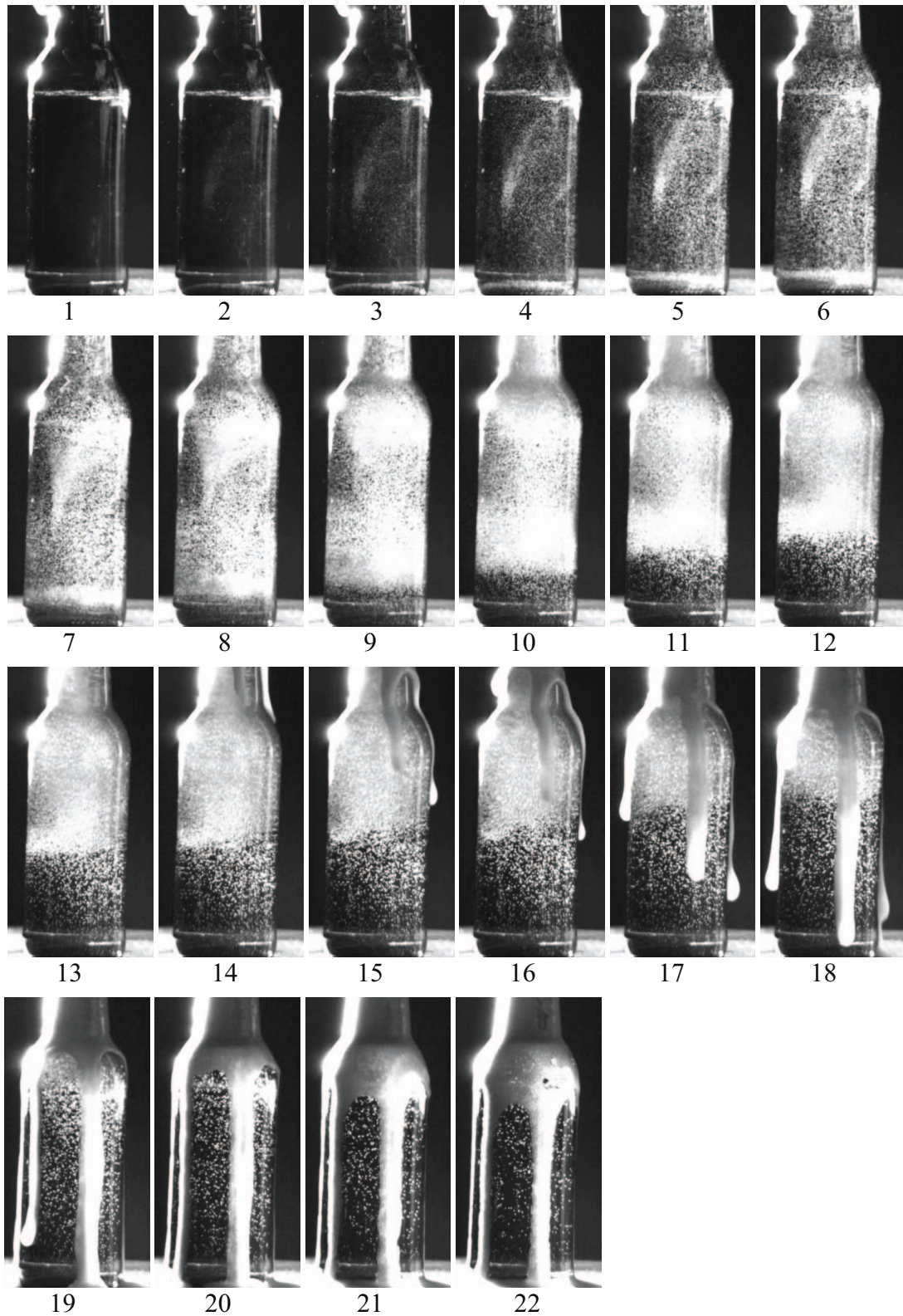
Figure 43 Snapshots of the multi-phase expansion of a gushing beer. The single frames were taken from short videos recorded by a high resolution camera of Bielefeld University.
