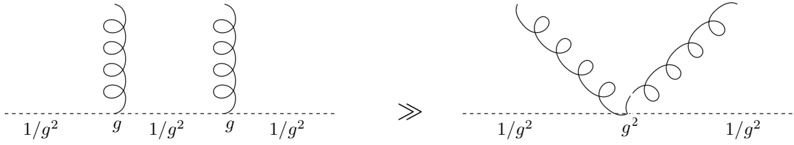
Figure 3.6.: Diagrams involving seagull vertices are suppressed compared to diagrams with only trilinear vertices because one propagator is 'missing' and cannot give a 1/g^2 enhancement. The same reasoning applies to four gauge boson-vertices.
