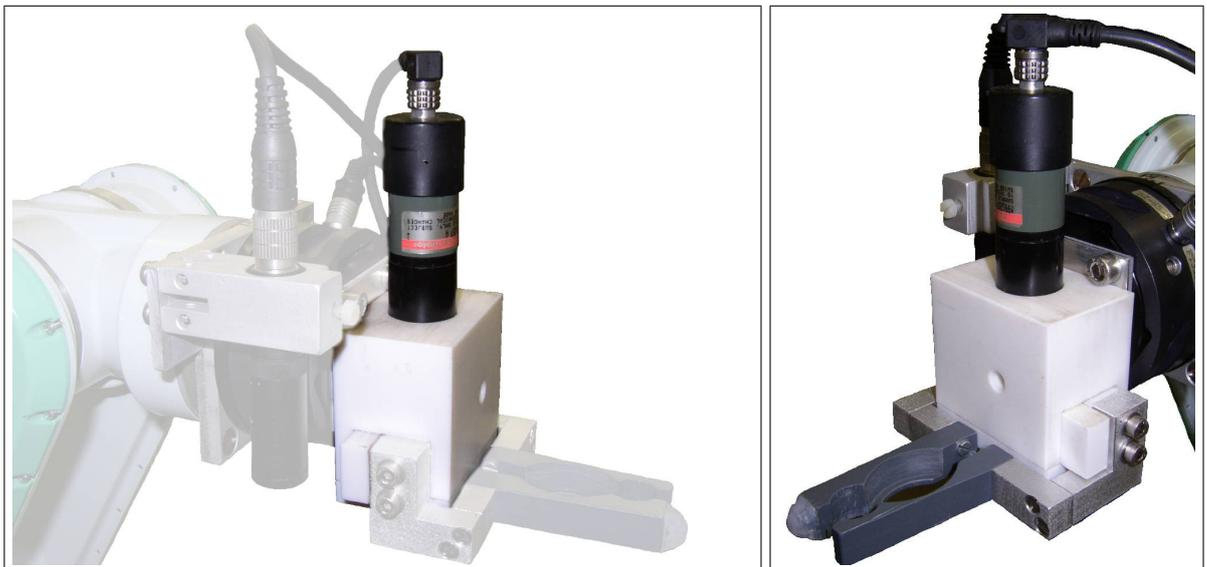
**Figure B.6:** The electric parallel yaw gripper.
