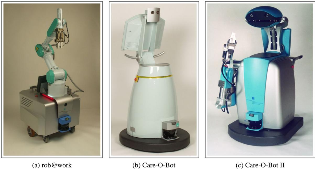
**Figure 1.7:** Three generations of service robots developed at the Fraunhofer IPA Institute.
