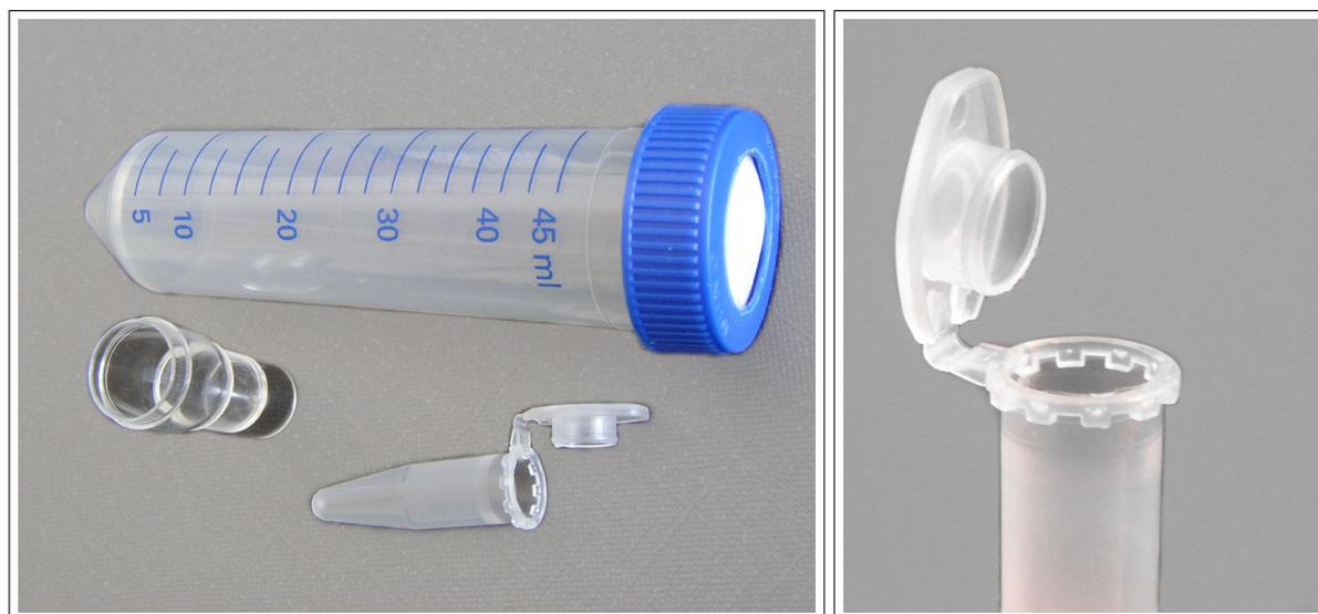
**Figure B.8:** Three different kind of tubes used for manual sample management. Left image: A 50 ml NUNC tube (upper), a 1 ml Cedex tube (lower left) and a 1.5 ml Eppendorf tube (lower right). Right image: A closeup of the Eppendorf tube.
