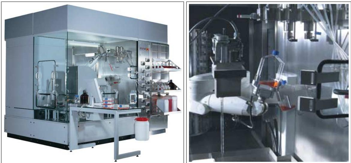
**Figure 1.5:** The “Select” automation workcell by The Automation Partnership using a standard robot arm. Images © by The Automation Partnership. <http://www.automationpartnership.com>
