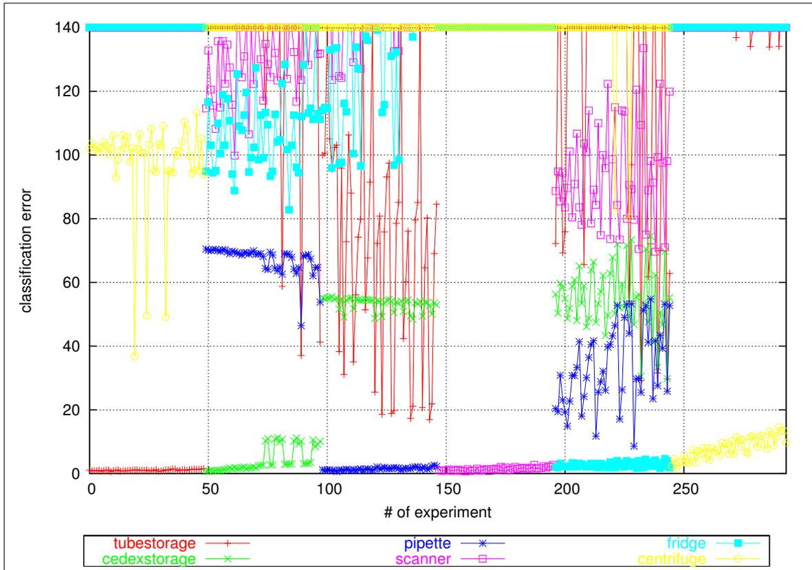
**Figure 5.37:** The classification error (MSE)  $e_{C,M}$  for six different objects in several different displacements in a  $24 \times 24$  millimetres grid. The experiments for each object are sorted according to an increasing absolute value of the displacement and the error has been clipped at 140.
