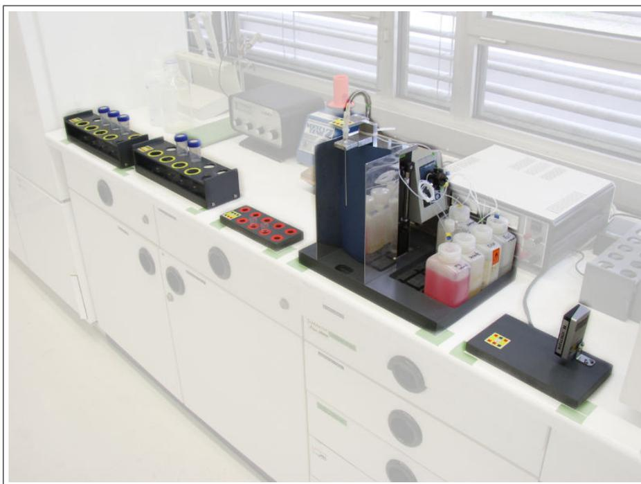
**Figure 2.4:** The pipetting device, together with some of the storage racks.
