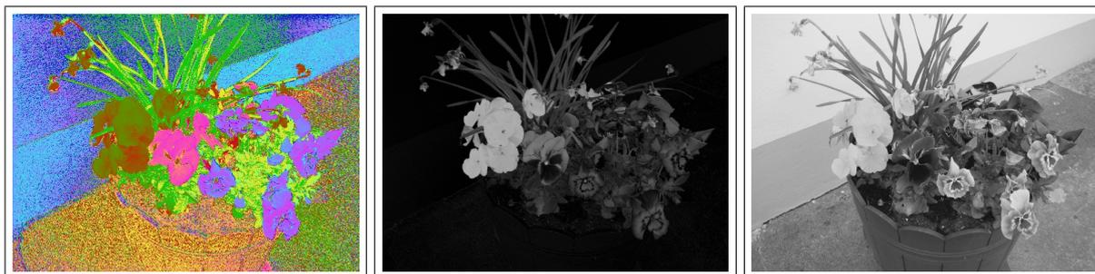
**Figure C.13:** Decomposition of the image in figure C.5 into (from left to right) the H (*hue*), S (*saturation*) and V (*value*) channels of the HSV colour space. All the channels are by definition greyscale images, but the H channel has been re-colourised for better visualisation.
