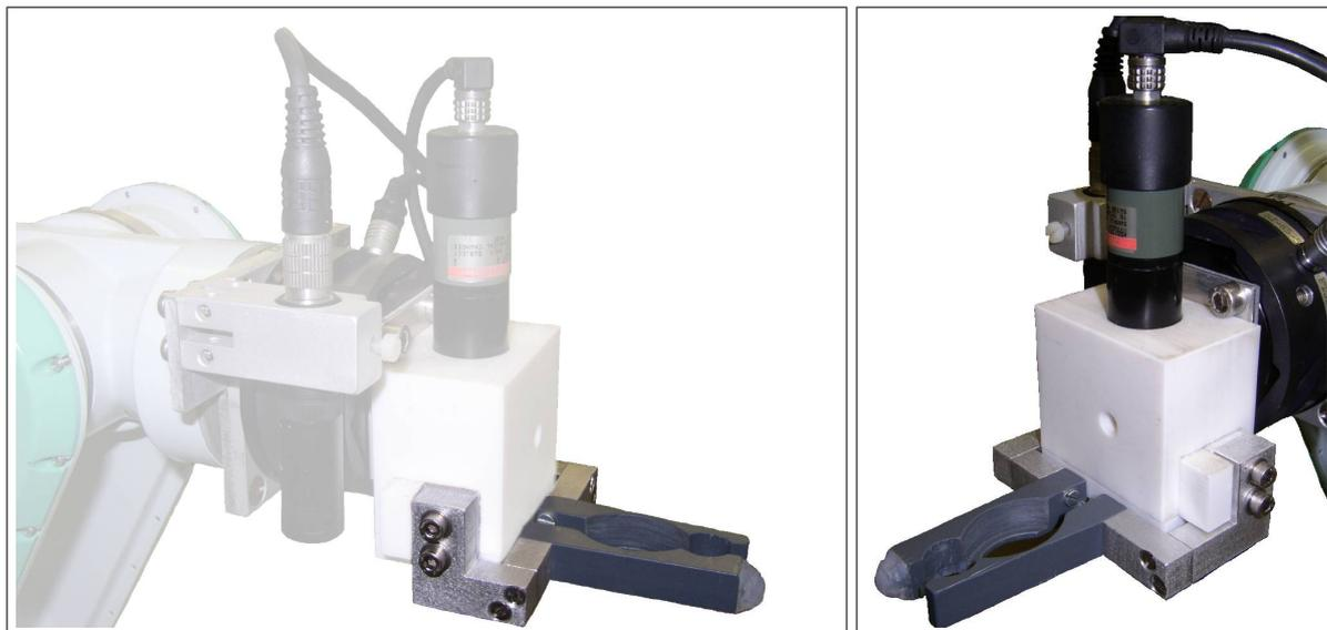
**Figure B.7:** The customised gripper fingers with curved cut-outs fitting the NUNC and Cedex tubes and a piece of silicone rubber to press buttons on the membrane keyboard of the centrifuge.
