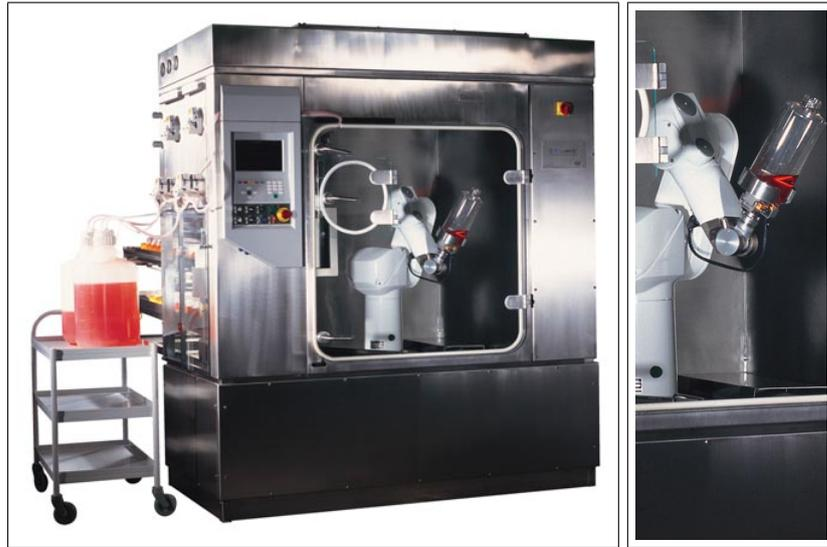
**Figure 1.4:** The “Cellmate” automation workcell using a standard robot arm. Images © by The Automation Partnership. <http://www.automationpartnership.com>
