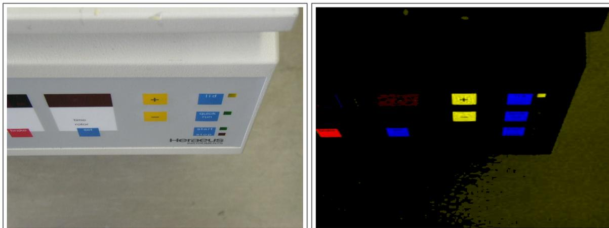
**Figure 5.17:** Visualisation of the information reduction by focusing on coloured regions. Left: original image of the centrifuge, right: reconstruction based on the colour similarities in figure 5.16.
