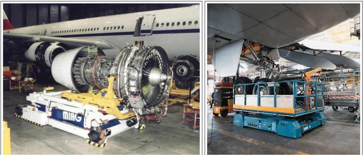
**Figure 3.1:** Autonomous guided vehicles by MIAG used in aircraft industry.
