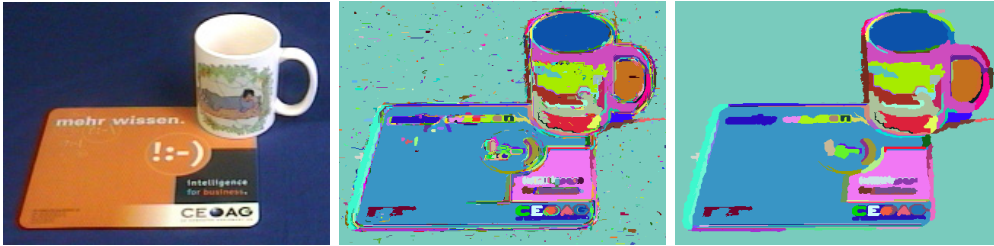
Figure 2.10: Example image from the office domain (left) and segmentation results delivered from the segmentation method proposed in [Felz 98]. Parameter settings are k=150 , s=0.8 . Results without accounting for segment sizes (middle) and with additional postprocessing using minimal segment size threshold m=64 (right).
