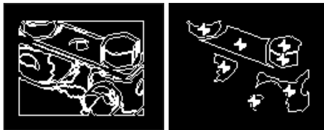
Figure 3.12: CSC color segments and selected segments that provide high color contrast and determine focus points for the example image of Fig. 3.9.
