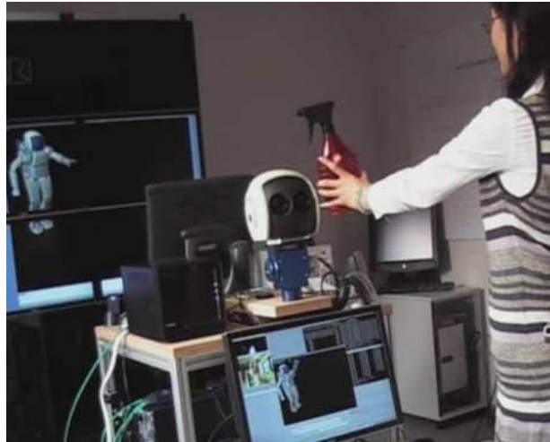
Figure 4.6: Give and show: experimental settings. The user shows an object to the camera head. The real camera moves and captures the images while the movement of the robot's hand is only simulated. The user can see the gesture displayed on a big monitor and decide how to react: give the object to the robot or only show it. The second monitor on the bottom is used to display internal states of the system for debugging purposes.
