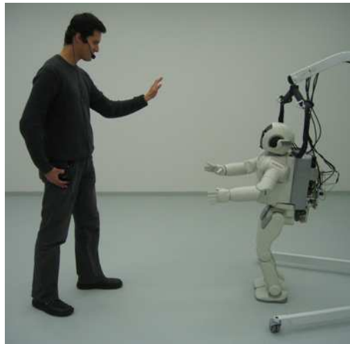
Figure 4.13: Experimental setup. The humanoid robot ASIMO interacts with a user in a reactive way by approaching and reaching for a proto-object. The user wears a headset for recording the speech signal. The user can teach the robot speech labels which describe behavior-relevant features of interaction: properties of proto-objects or the activity of the robot.
