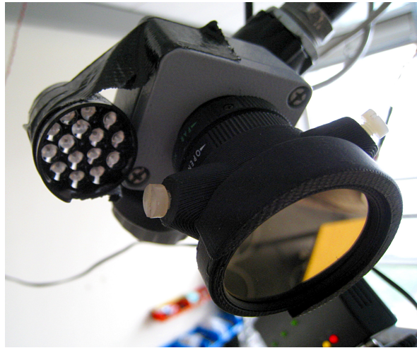
Figure 10: One of the cameras SCOTTY uses. To the left the LED array can be seen that projects infrared 880 nm light along the camera's optical axis. Right in front of the camera a band-pass filter is mounted with a fitting manufactured by C5 student assistant Alexander Neumann using a 3D printer.
