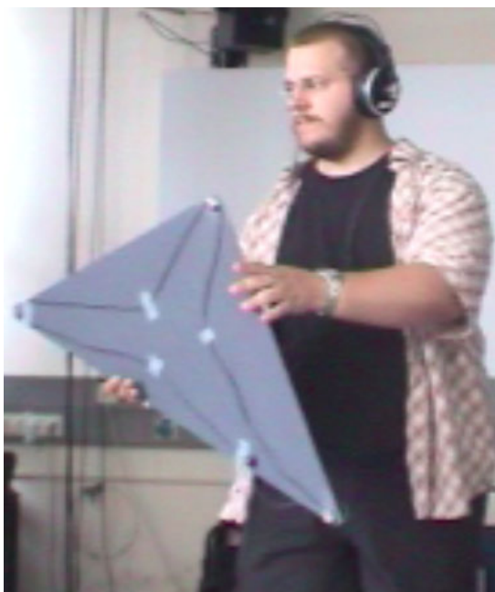
(a) Tangible Data Scanning Sonification. The photo shows a user with an interaction tool, scanning the data cloud in data space that has been identified with the physical space. Headphones plus headtracking allow convincing spatial perception of intersection events.
