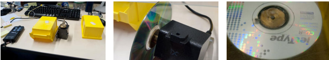
(a) Overview of the measuring installation. The step motor for controlled movement of the magnet and two yellow boxes on which the CTI is placed during measurement. (b) A CD attached to the step motor served as a fixation for the measuring magnet. (c) Magnet connected to the CD.
