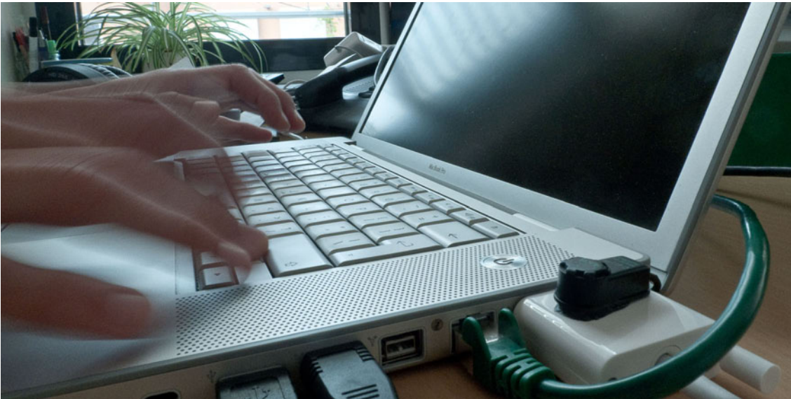
Figure 9.30.: The hardware setup used by Participant 1. The transducer was attached to the external video adapter of her laptop. This made it easy for (dis-)assembly, since she only used WetterReim at her workplace, but carried her laptop with her.
