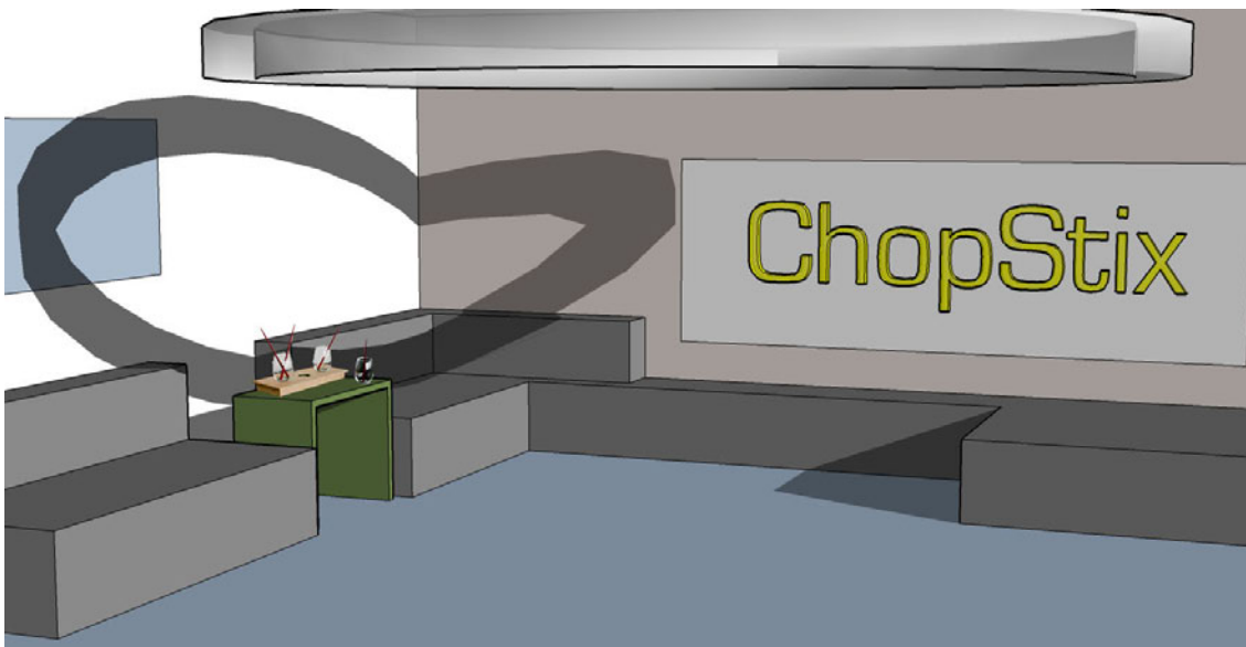
Figure 9.19.: A rendering of the location of the ChopStix Interface in a room. The spatial sound display is realised by the ring of loudspeakers on the ceiling. The long-term aspect in the control – near real time data streams change their values on an hourly basis – requires the interface to be constantly available, but not to be disturbing. Therefore it is placed near the edge of the used multi-speaker setup.
