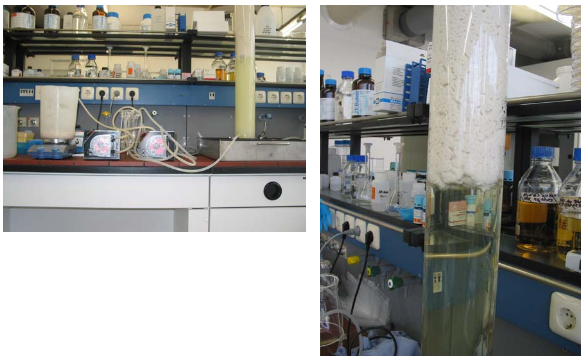
Figure 25 Scale up of alkaline lysis and neutralisation using a flotation column.
