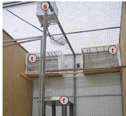
Fig. 1: Mate choice set-up. Choosers flew freely within choice aviary after start box (s) was opened. f = food & water, t = test cage with subjects.
