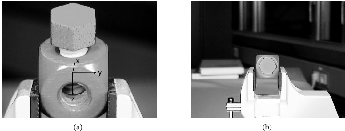
Figure 5.1: A screw-cube assembly under two different image scales and perspectives. a) The assembly is perceived under a 60^\circ elevation from the yz -plane of the depicted coordinate system that is attached to the cube. The image scale is 0.1mm per pixel. b) The same assembly, perceived under an elevation of 0^\circ and an image scale of 0.3mm per pixel
