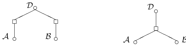
Figure 4.2: Component \mathcal{D} is the smallest component that contains components \mathcal{A} and \mathcal{B} . Left: \mathcal{D} is on the path between \mathcal{A} and \mathcal{B} . Right: \mathcal{D} is not on the path between \mathcal{A} and \mathcal{B} .
