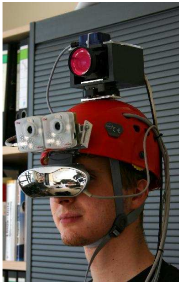
Figure 8.1.: The assistance system: Hardware setup of the AR gear. It has been designed and assembled by Graz University of Technology [SP04].
