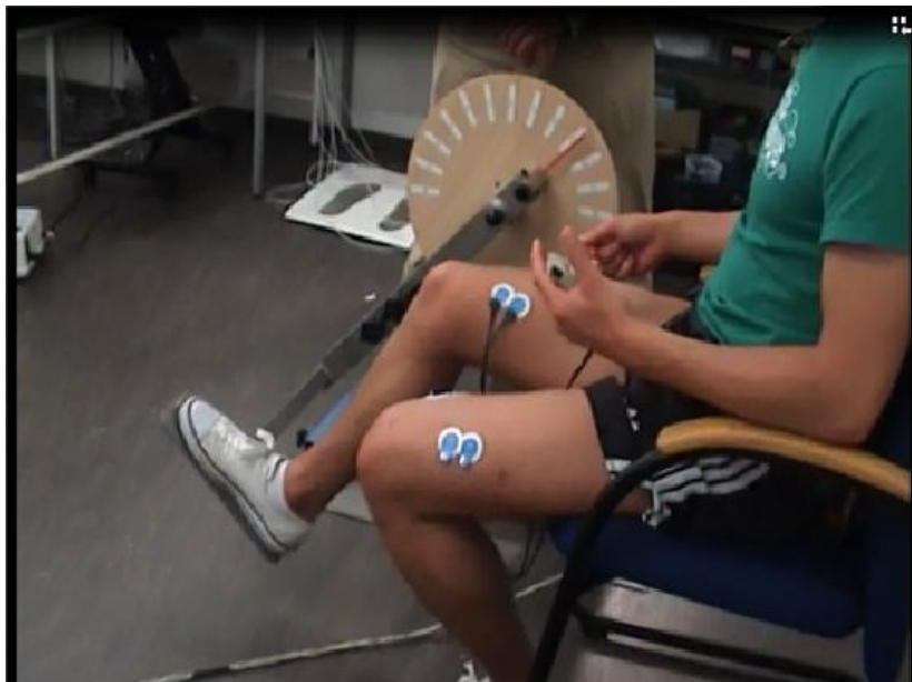
Figure 3. Recording of EMG of muscles in different angles
