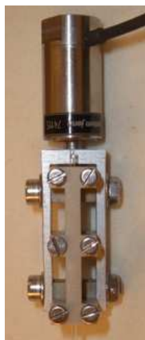
Figure 4.12: Photograph of the piezo stack actuator with the pipette holder attached.
