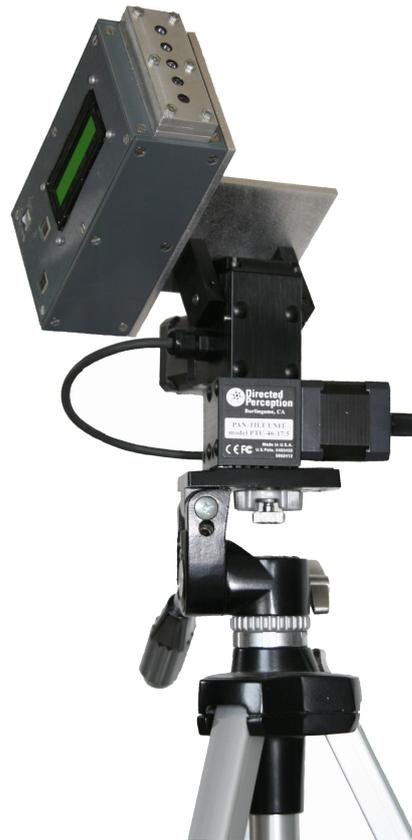
Figure 6.6: 2-D pan-tilt sensor, a combination of a Directed Perception pan-tilt unit (PTU-46-17.5) and the five-channel handheld sensor.
