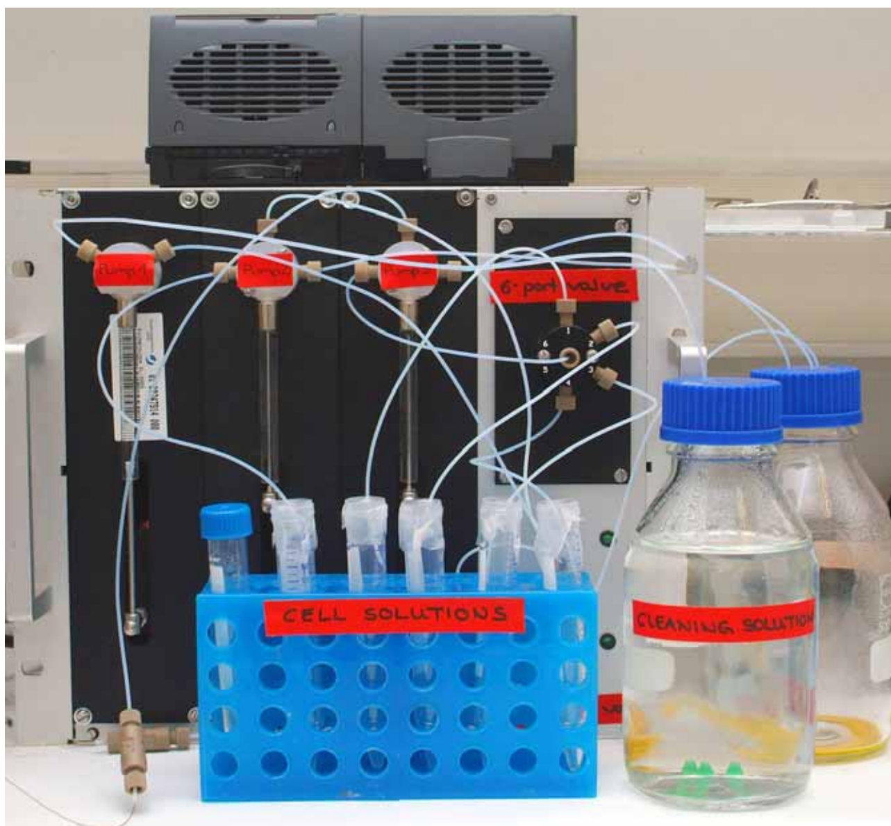
Figure 3.78: An analogue pump station was assembled in Jülich: The SV 6-port valve is to the fore, whereas the inert valves cannot be seen.
