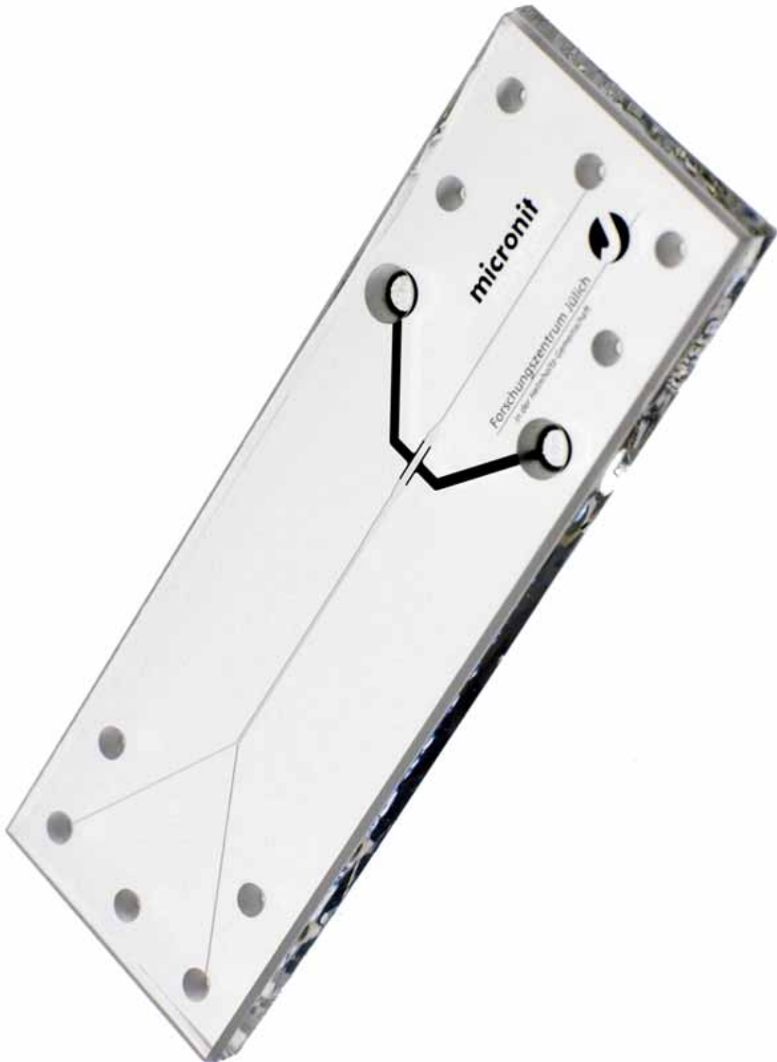
Figure 3.119: Reduced version of the microfluidic electrofusion chip for the study of the fusion process of mammalian cells.
