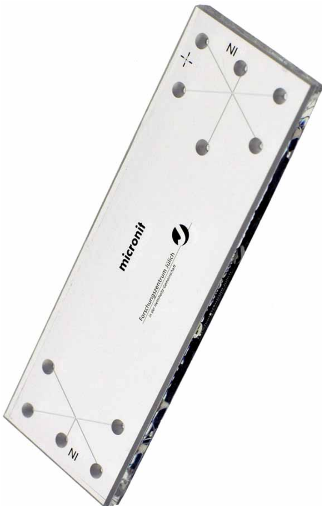
Figure 3.120: Splitter chip for the use with the microfluidic electrofusion chip to reduce the number of required pumps from nine to two.
