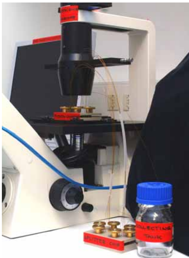
Figure 3.124: The electrofusion chip with chipholder can easily be placed on an inverted microscope, whereas the splitterchip can be placed elsewhere.
