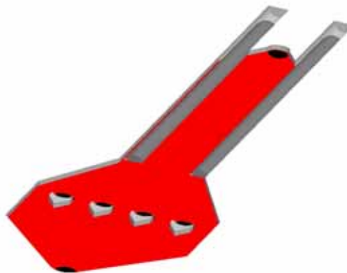
Figure 3.110: Sketch of the microfluidic system 3 with positioning of two Platinum wires as electrodes alongside the microfluidic chamber
