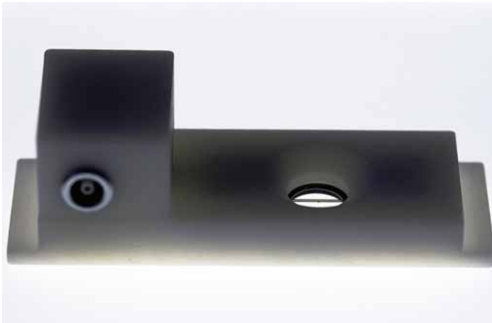
Figure 3.1: Micro fusion chamber for the Eppendorf Multiporator: It consists of a casing containing two electrodes above a transparent reservoir. Connection to the Multiporator can be established by a coaxial cable via a special insert. This micro fusion chamber allows the optimisation for cell alignment and cell fusion under microscopic control.
