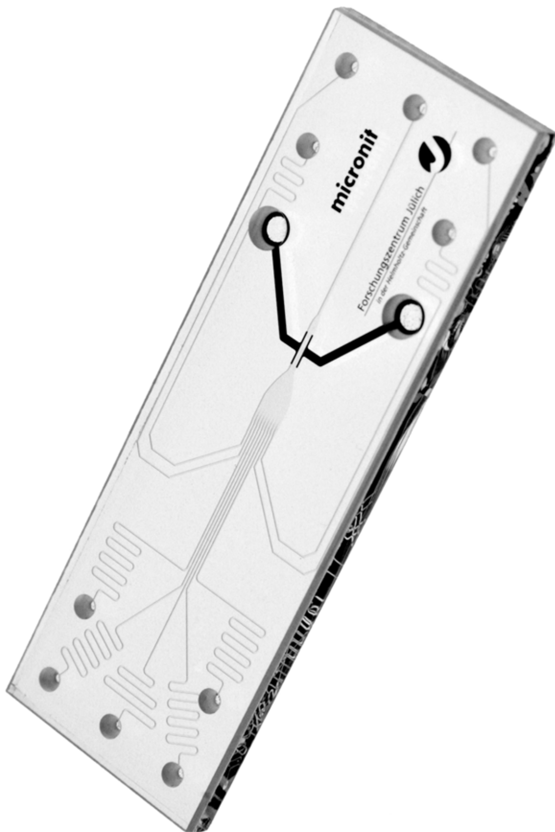
Figure 3.118: Microfluidic electrofusion chip with nine inlets, one outlet and two electrodes (with feed line to contact patches) alongside the rear part of the chamber for the generation of large numbers of hybrids.
