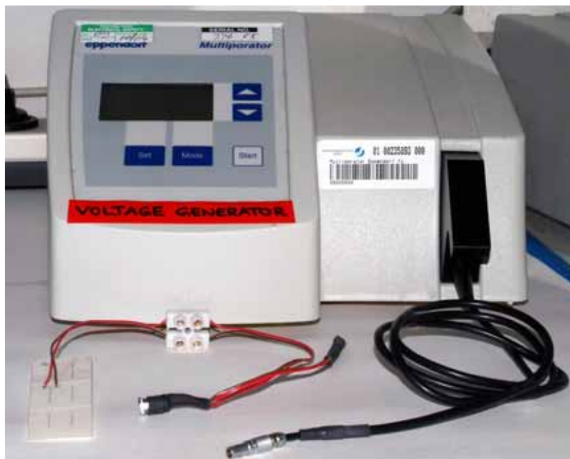
Figure 3.43: The completed electrofusion chamber can be connected via a push-pull self-latching connection system to the voltage generator from Eppendorf.
