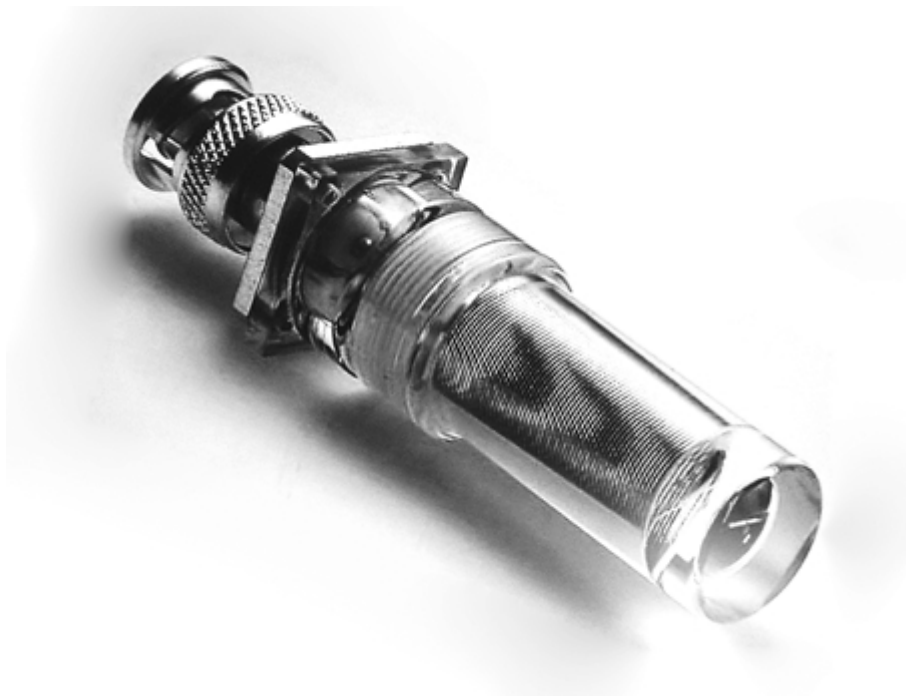
Figure 3.3: Helix chamber for the Eppendorf Multiporator: It consists of a conical core that carries the parallel wrapped electrode wires and a beaker into which the cell suspension is added. The filling volume accounts to 250\mu L . The electrode gap width of 200\mu m is filled by the screwing of the core into the beaker, whereupon the cell solution is pressed upwards into the gap.
