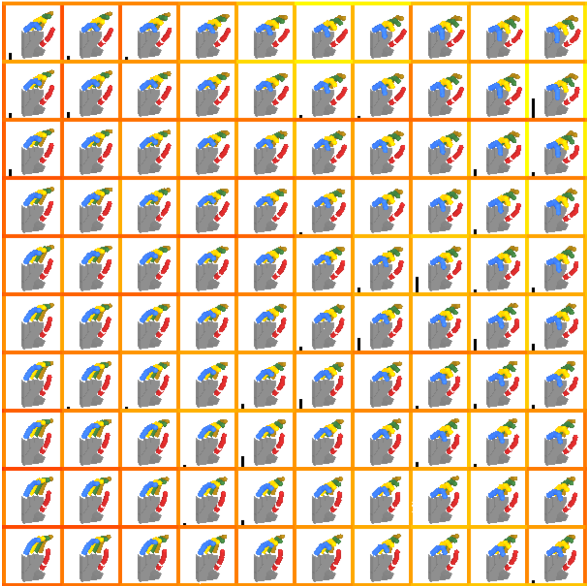
Figure 4.8.: 10x10 extract of the cylinder-specific 25x25 SOM Grasp Manifold used for Figure 4.3 and Figure 4.4 after resuming the learning with grasp postures generated by the experience-based grasp control. The node structure is now very smooth, the hand postures fade smoothly from one node to the next.
