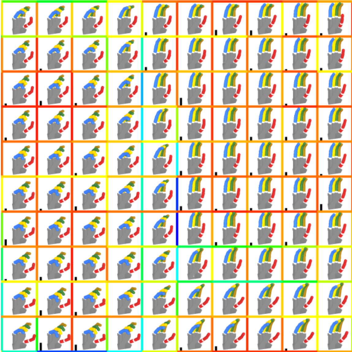
Figure 4.3.: 10x10 extract of a cylinder-specific 25x25 SOM Grasp Manifold . Each hand posture visualises the reference vector \mathbf{w}_a of one SOM-node. The smooth changing of the postures supports the assumption of the Grasp Manifold . The colour of the sub-figure borders encode the inter-node distance (red: minimal distance, green: medium distance and blue: maximal distance). Black bars left from the hand indicate the relative amount of training data that support the corresponding SOM node; no bars indicate the lack of supporting training data.
