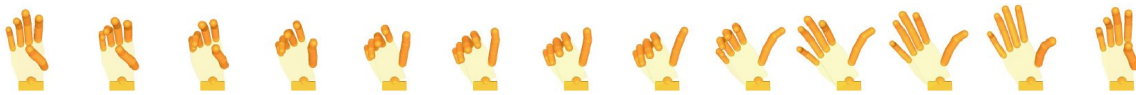
Figure 5.1.: Visualisation of an exemplary sequence of a recorded cap turning manipulation movement. The illustrated hand postures are generated in a physics-based simulation, controlled via a data glove. Joint angle corrections are incorporated from the collision detection module of the simulation software which avoids a penetration of the fingers and the bottle cap, that was present in the recording scene.
