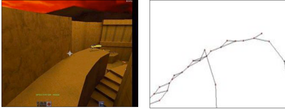
Figure 5.1: A screenshot of a small part of the map and the corresponding waypoint map
