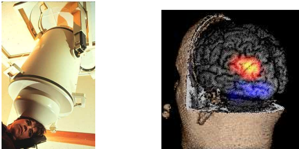
Figure 1.2: Left: BTi 37 channel probe biomagnetometer (Biomagnetic Technologies, USA). Right: Magnetic field over the brain, 0.15 seconds after display of a moving visual stimulus. The yellow/orange region indicates where the magnetic field is strongest.
