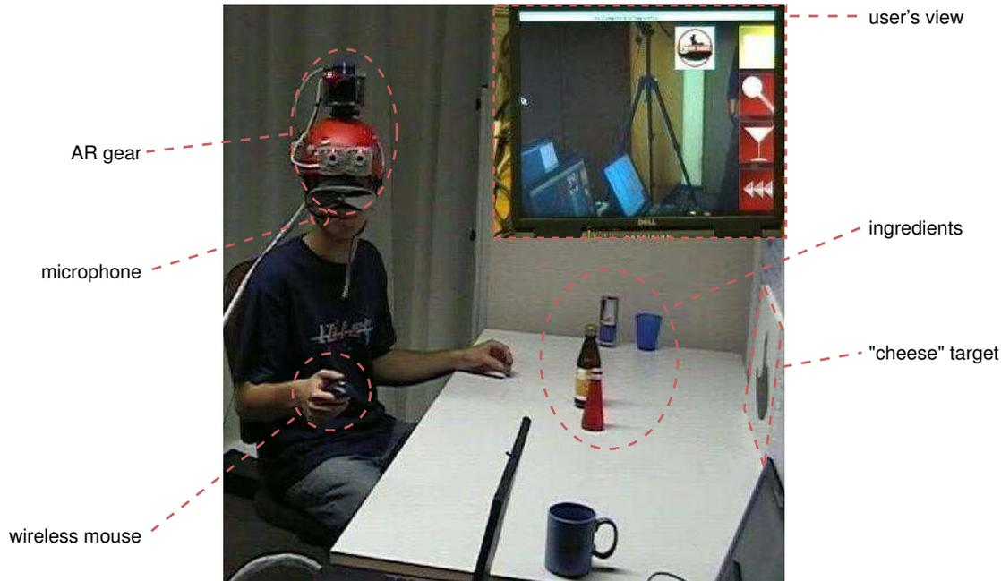
Figure 8.13: Experimental setup for the user studies: Subjects have been recorded during the evaluation sessions from this perspective for analysis.
