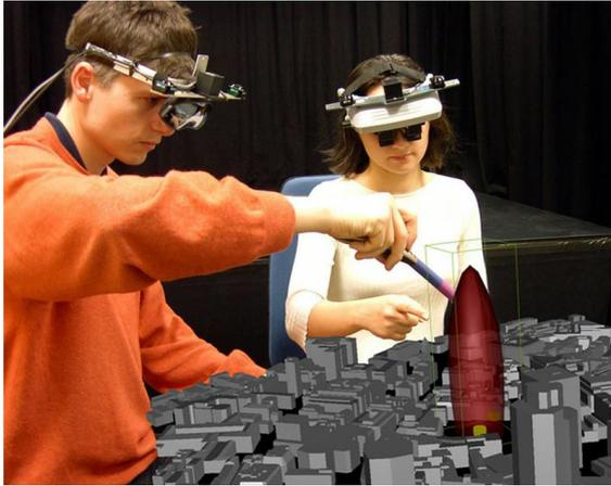
(a) An augmented reality system for architectural design (© ARTHUR-System, Fraunhofer Institute).
