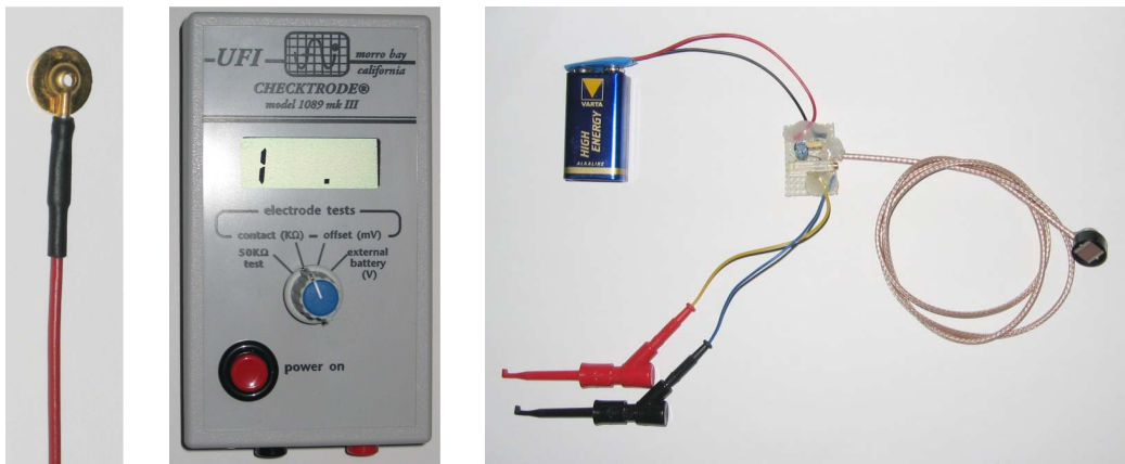
Figure 7.4: Left: Gold cup (Au) electrode as used in the experiment in this chapter. Middle: Checktrode 1089 mk III electrode tester for assessing impedances. Right: Circuit with an adjustable photo resistor for measuring temporal relationships between screen presentations and EEG recordings.
