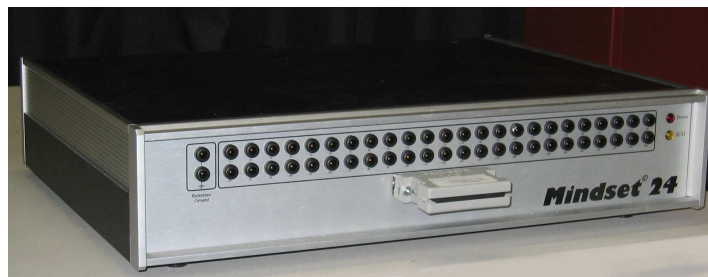
Figure 7.3: The Mindset24 EEG amplifier with 24 differential input channels.
