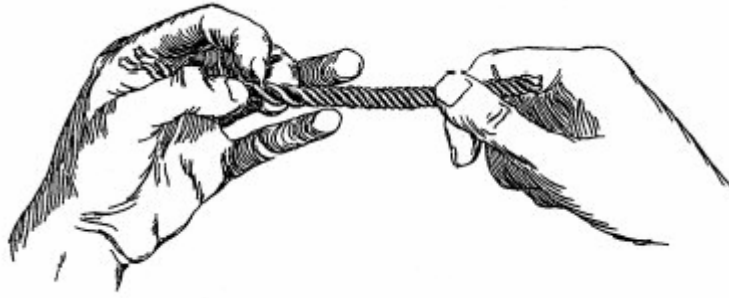
Fig. 3. The screw sensed on a rope (right) and the nut sensed by the finger nails (left).
